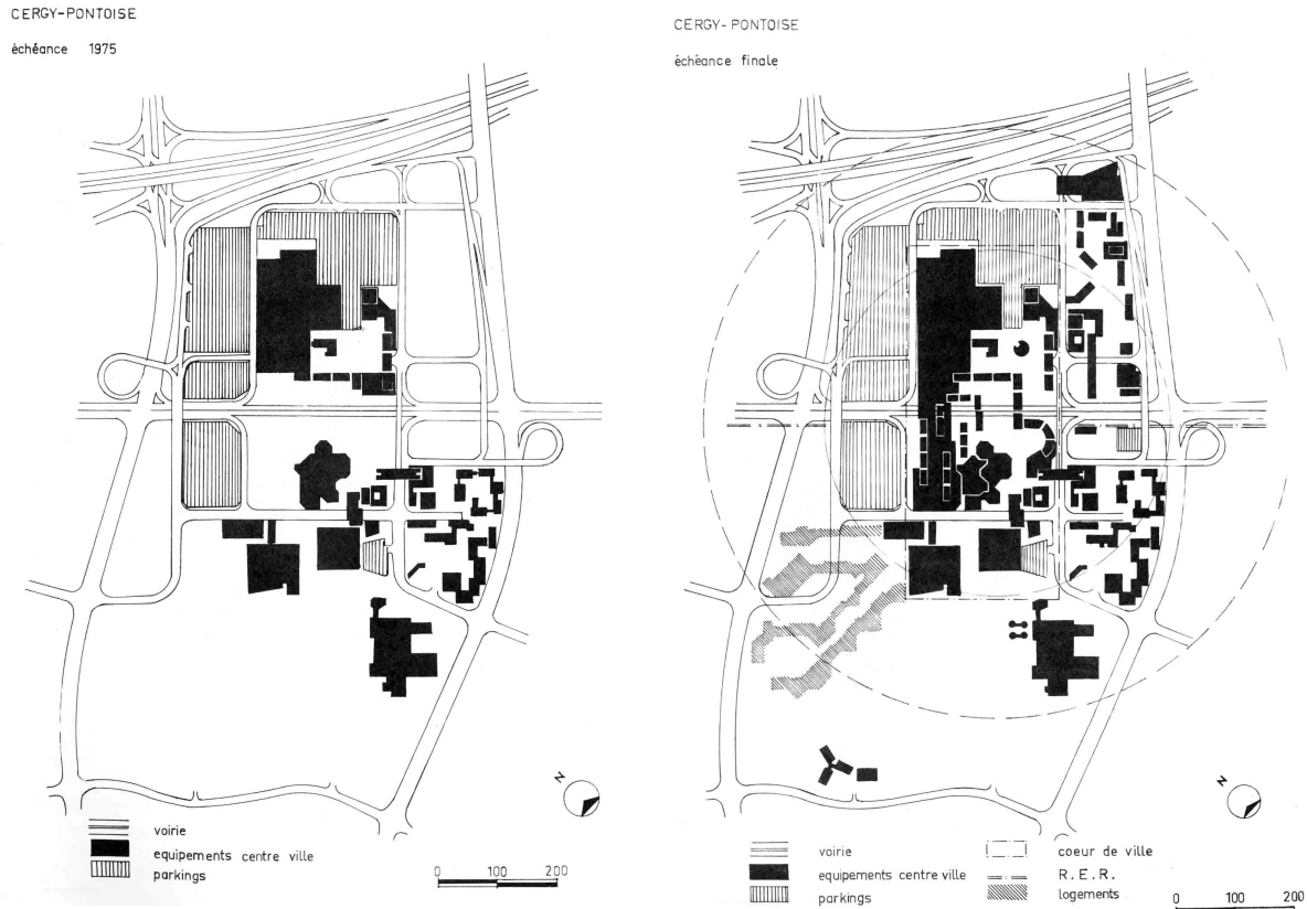
Figure 5.18: Diagrams for the urban center of Cergy, drawn in 1972 by the architect Aymeric Zublena, showing how car circulation and parking defined position and integration of shopping mall with other functions, with construction phased over time (Source: Amercio Zublena, Patrice Noviant, and Xavier Triplet. “Les centres urbains des villes nouvelles françaises,” (Paris: Ministère de l’Equipement / SGGCVN, 1972): 22-23 (CDU)).
